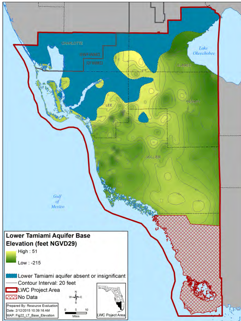
Figure 22. Elevation of the base of the Lower Tamiami aquifer.
